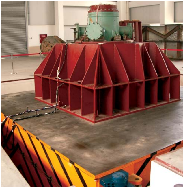
Figure 1. 6 meter x 6 meter seismic table with eight actuators – 4 Z, 2 X, 2 Y.
